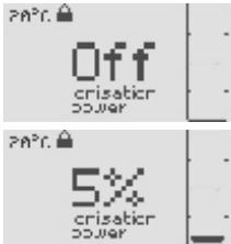
ATTENTION: First install the pump and activate the water supply, before connecting the display unit. Set the ionisation power at 5% activation. Wenn the water flow is not running, the message appears: ERROR 1.
